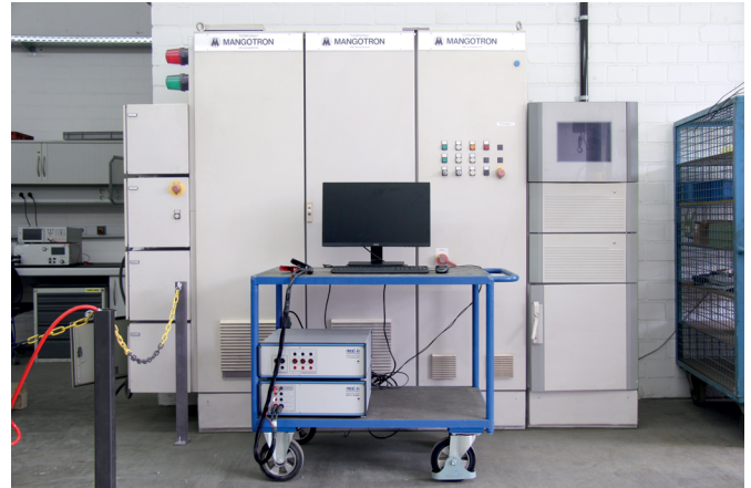
Figure 5: Control cabinets of the DC linearity test bench in the background, in front trolley with DPG10-4000B/F and PC
